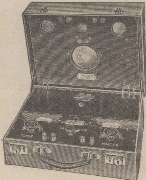
The "Rolls" portable, a handsome three-valve model exhibited by Messrs. Detex Distributors. The frame aerial and loud-speaker are built into the lid.
