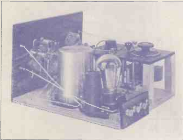
This back-of-panel photograph shows the placing of the various components, such as the Screened Coil, High-Frequency Choke and the Integral Wave-Trap. The design is one which will commend itself to many.
