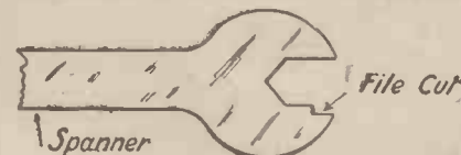
Fig. 1.—A thin flat file should be used for making the cut in the spanner.
