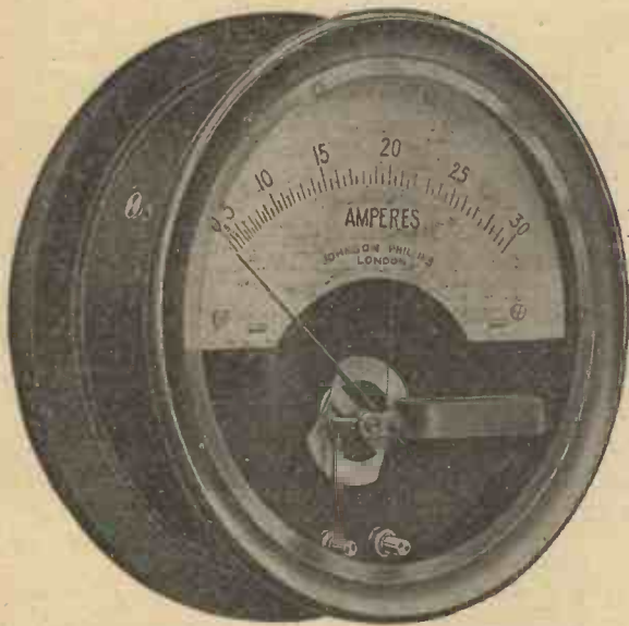
A well-known form of hot wire ammeter.
