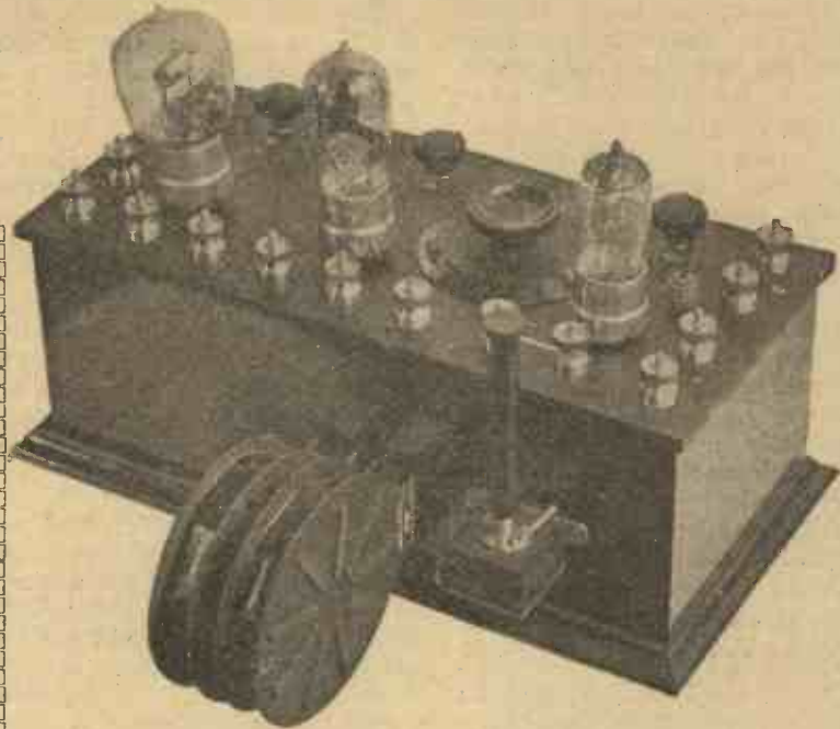
In this amplifier, described in "Wireless Weekly," Vol. 4, No. 14, plug-in coils are used for the anode and neutrodyne circuits.
