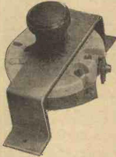
A filament resistance of this type is easily fitted for experimental work.
