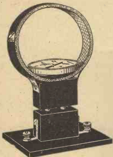
Fig. 1.—The galvanometer may be mounted upon a stand made from a coil socket and a small piece of ebonite.
