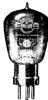
The Mullard D.F.A.A. valve, a type of valve suitable for resistance amplification.
