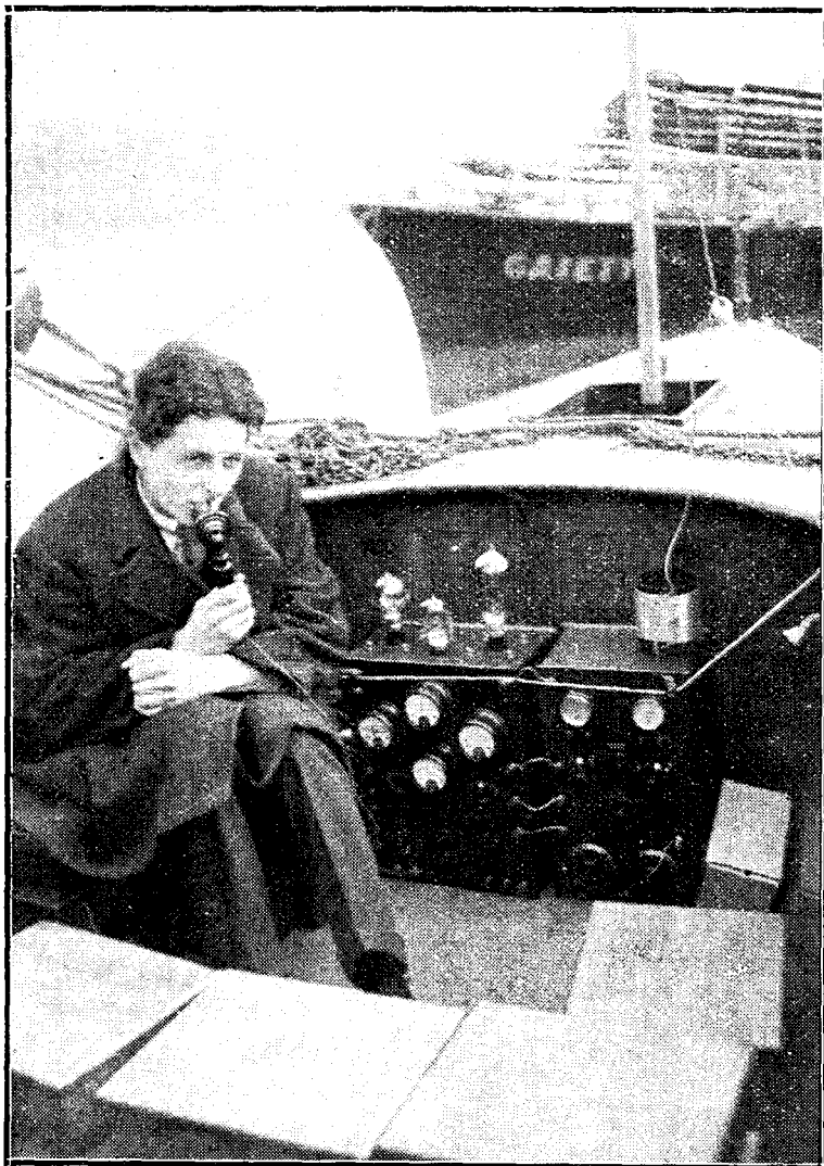
Capt. R. Tingey testing the transmitter. Note the aerial inductance referred to in the article.
