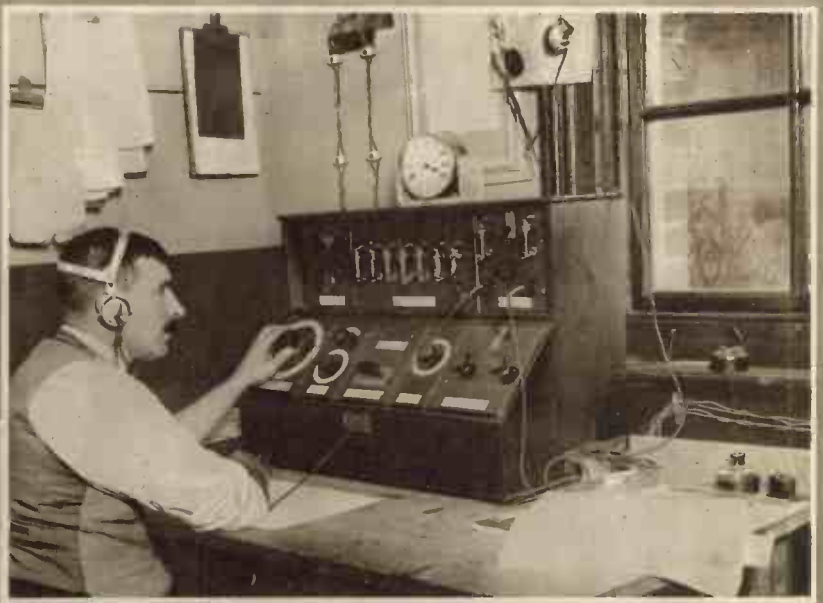
A new wireless directional station on the southernmost point of the Isle of Wight, at Niton, will be in operation before winter fogs become a menace to ships constantly using the Channel. The new station at Niton will be able to communicate with ships in any of the Channel waters, and will enable them to find the exact spot over which they are steaming. A five-shilling fee is charged for each direction. On the left: Leading-in wires of the D.F. aerial.
