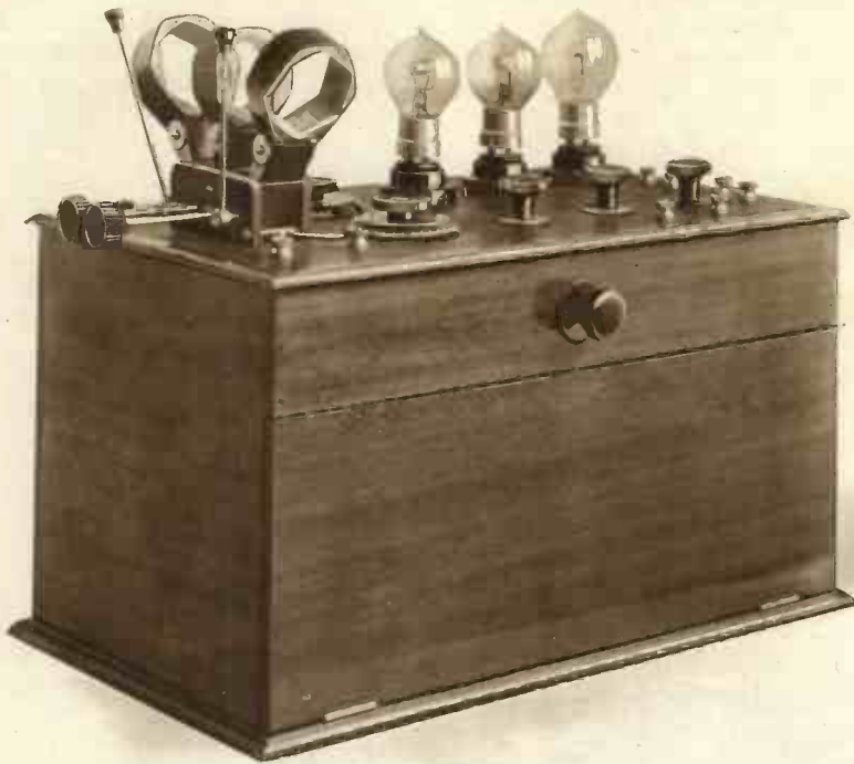
Fig. 1.—The batteries are carried in the cabinet beneath the apparatus.
