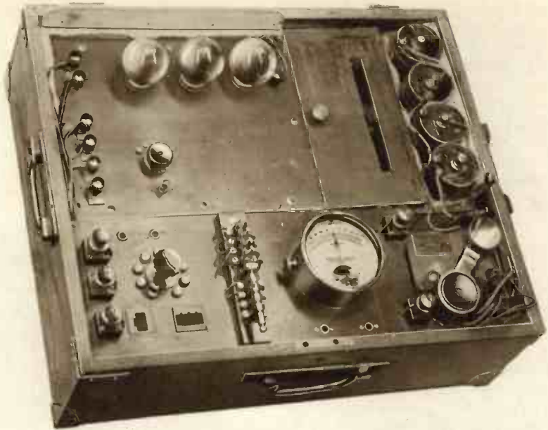
Fig. 6.—A special amplifying unit which is used for outside broadcasts.
