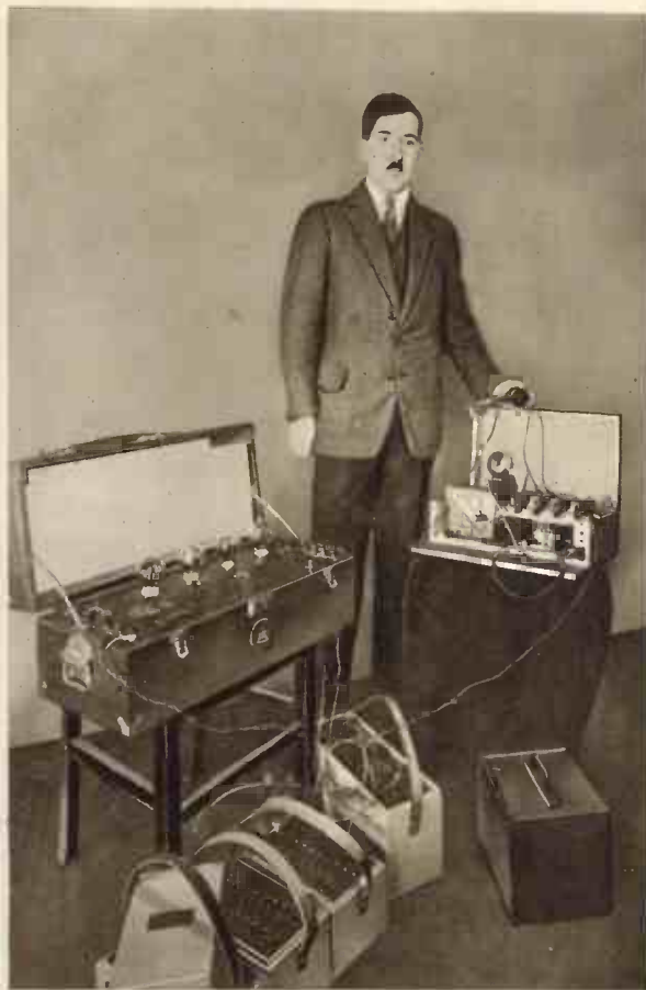
Fig. 4.—The amplifying apparatus for use in concert halls and theatres.
