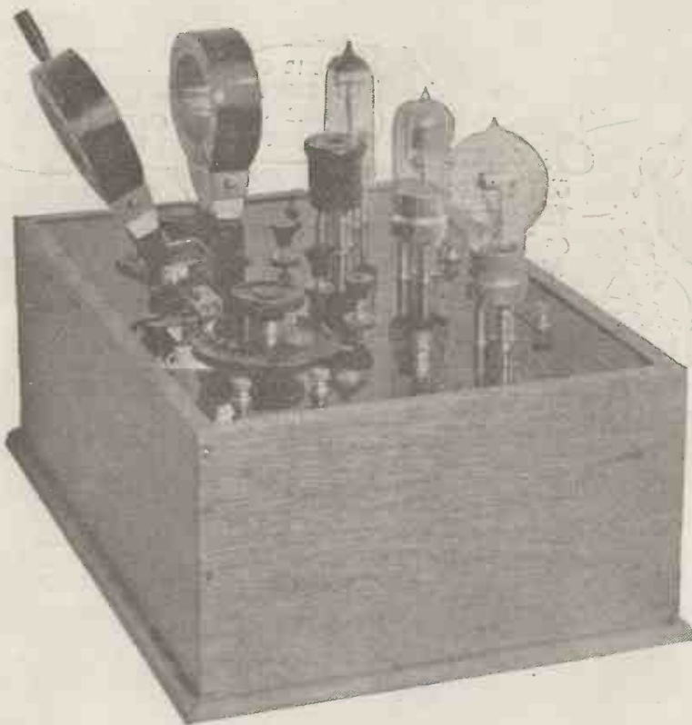
The receiver complete with valves, H.F. transformer and plug-in coils.
