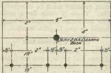
Fig. 45.—Lay-out of the panel.
