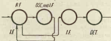
Fig. 1.—Showing how the signals are amplified at radio frequency. R.F.=Radio Frequency. I.F.=Intermediate Frequency. OSC.=Oscillator Valve.
