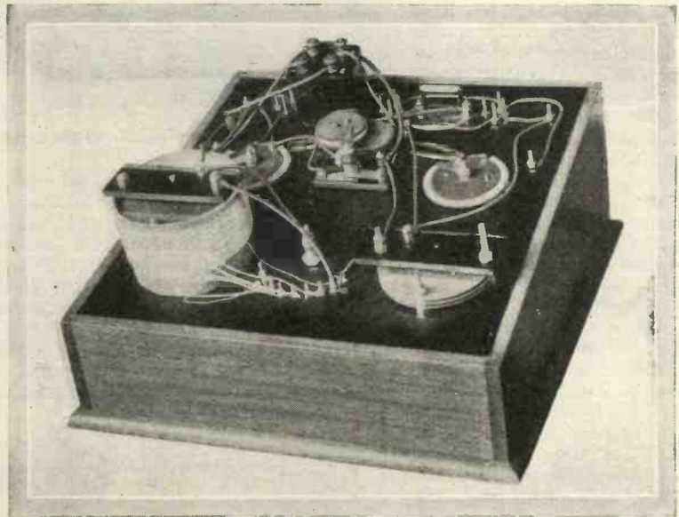
Fig. 6.—A back view of the panel showing the arrangement of components.
