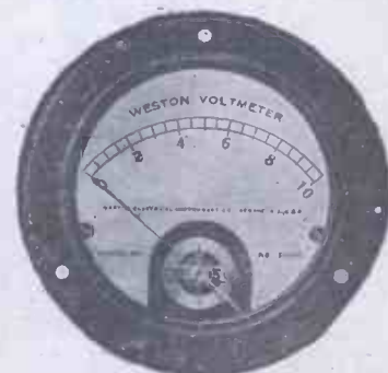
For accurate reading, a voltmeter having a high resistance should be chosen.
