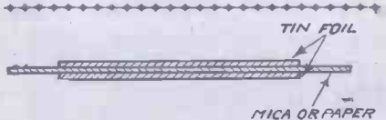
Fig. 1.—The elemental condenser unit referred to by the author in his discussions.
