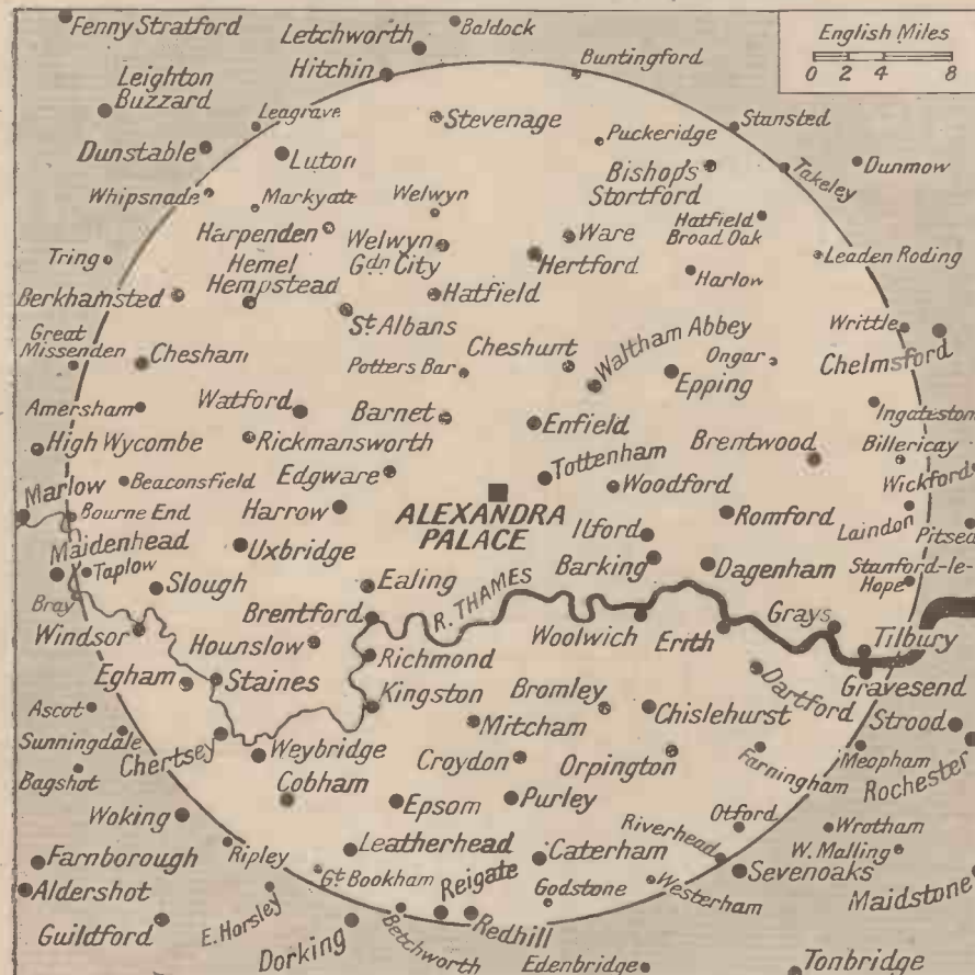
The choice of the Alexandra Palace for the London television station enables a very well-balanced area to be covered, as is shown in this map. About 25 miles radius is stated to be the real service range of the transmissions, and the circle shows the limit of this radius. It is probable, however, that places outside the circle will in many cases obtain perfectly satisfactory reception.
