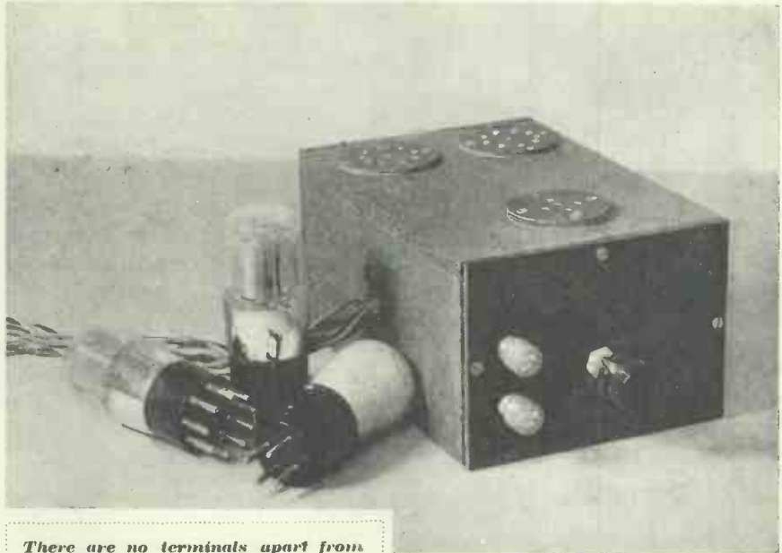
There are no terminals apart from those for input and output, the leads for the batteries being brought out at the side of the case. These can be seen behind the valves in this photograph.
