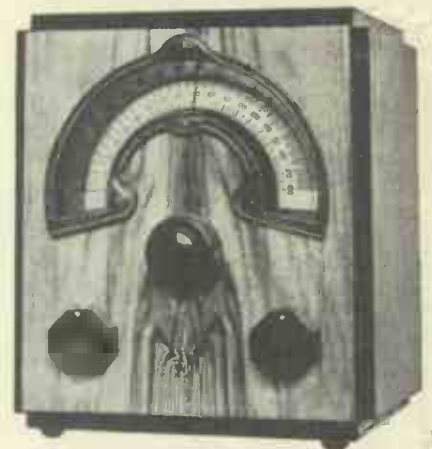
A Unit Radio instrument costing £2 10s. and having a range of 13 to 70 metres.
