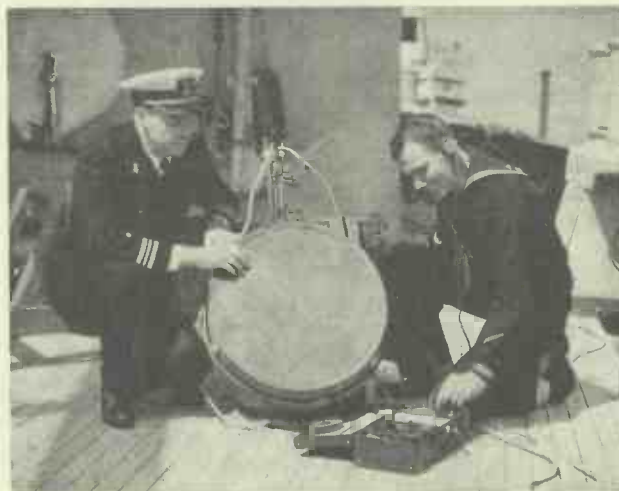
By changing sounds heard under water into electrical currents, this apparatus known as the hydrophone assists in the accurate determination of distance below the sea.
