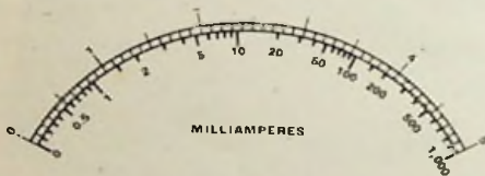
Fig. 29 : Scale of rectifier-shunted milliammeter compared with original to show the great increase in range of current measurable without shunting
