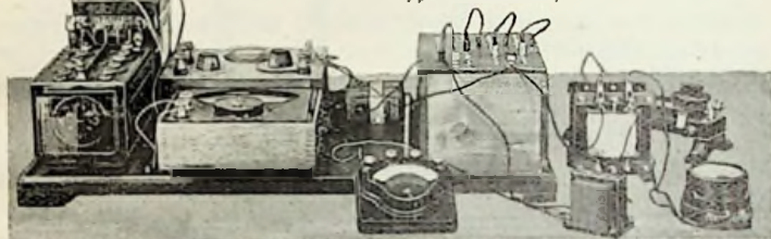
Fig. 3: The "quick hook-up"—the most temporary form of apparatus assembly
