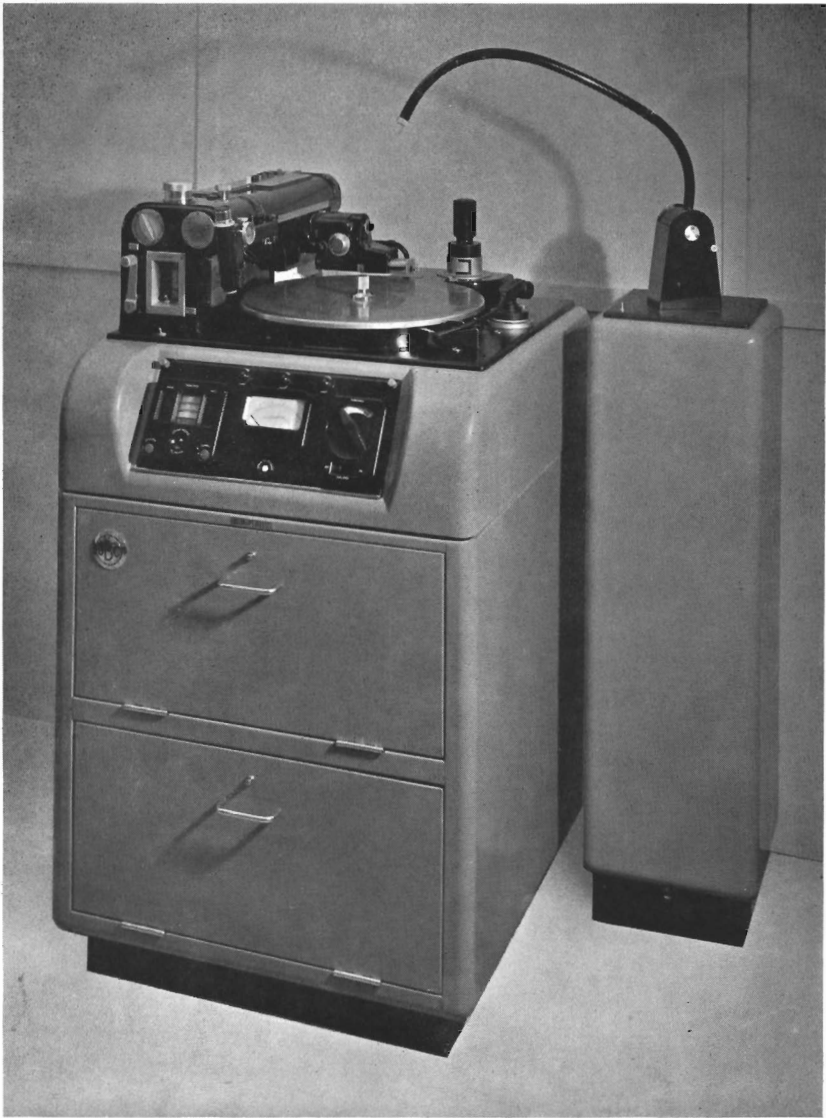
BBC disk recording machine Type D with swarf remover. Amplifier and mains unit are housed within the cabinet behind the flaps
