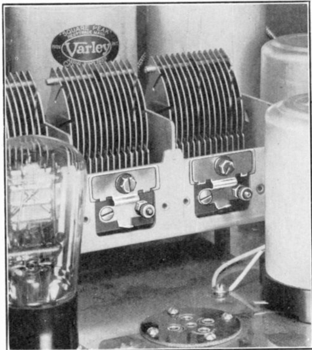
The layout is so arranged that there is easy access to the trimmers on the ganged condenser members. The oscillator trimmer is behind the valve in the foreground.
