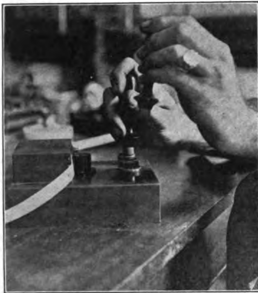
Perforating the tape for the transmission of wireless messages to ships at sea.
