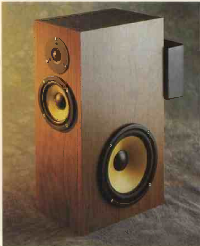
Due to the electronic bass-driver compensation, this full-range loudspeaker has a -3\text{dB} point of 25\text{Hz} . Response is \pm 3\text{dB} over the whole 25\text{Hz} to 20\text{kHz} range while power handling of the bass unit is 70\text{W} continuous.
