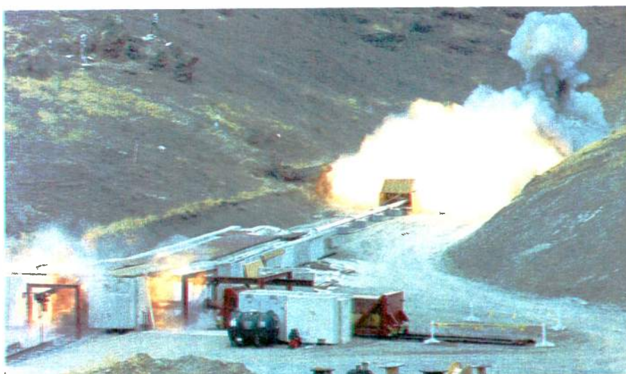
Supersonic launch from a light-gas gun, right and a projectile – a scramjet – in flight at Mach 8 just before entering a retaining bunker, above. In-flight glow is caused by the engine's hydrogen fuel and air friction. Flames on the right are hydrogen used to accelerate the jet along the 4in launch tube.
