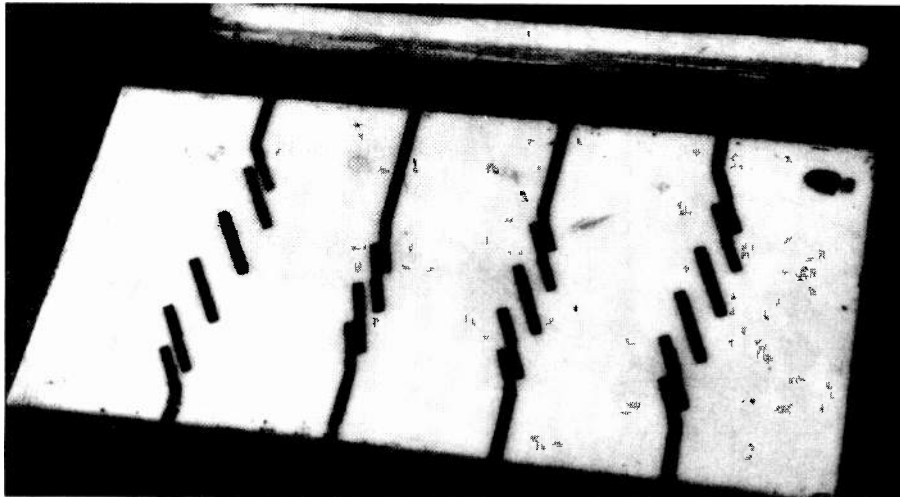
Fig. 3a. Four designs of an 18GHz microstrip bandpass filter on an alumina substrate. The length of each short section of line is approximately \lambda_g/2 and the amount of overlap between adjacent lines is \lambda_g/4 .
