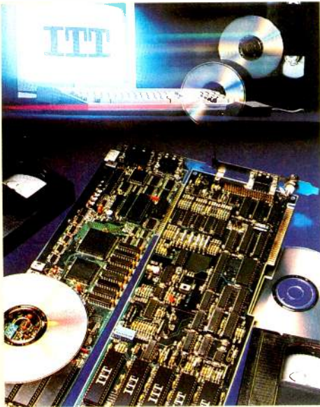
NTSC to VGA conversion: ITT's digital TV components perform a TV to computer display conversion for multimedia. The video adaptor uses an NTSC comb filter chip, the DPU2554 deflection processor, progressive scan processor PSP2210 and video codec VCU2134.
