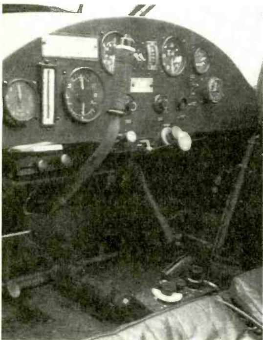
The Auster was normally used for spotting artillery, but the SOE had them fitted with the S-Phone (in front of seat).
