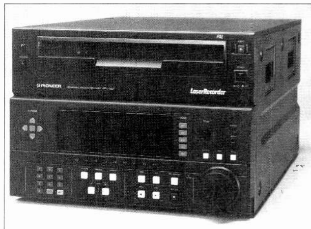
Pioneer's LaserRecorder is claimed to be the first rewritable videodisc recorder that conforms to the pal TV format.
