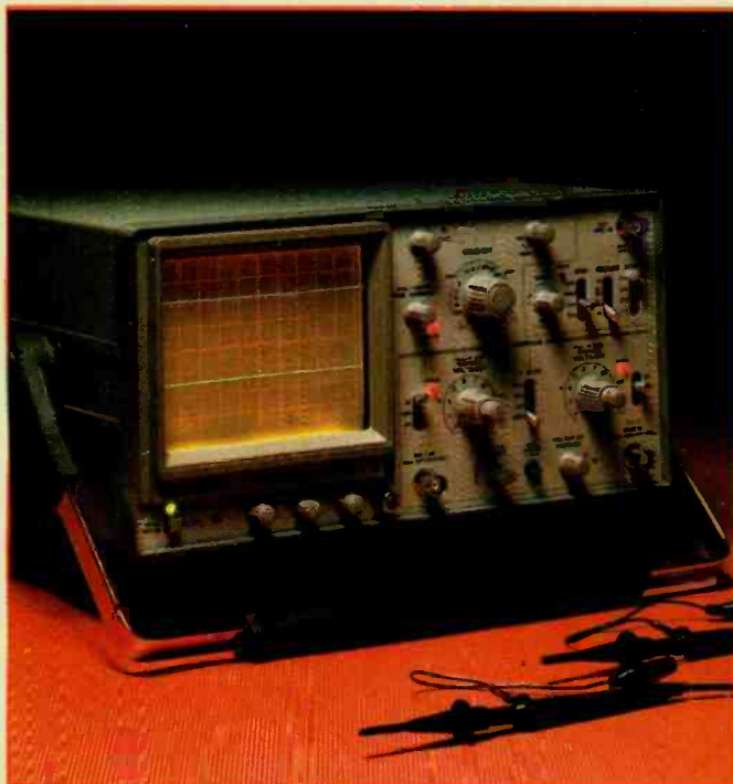
1021 general purpose oscilloscope from Leader Electronics
