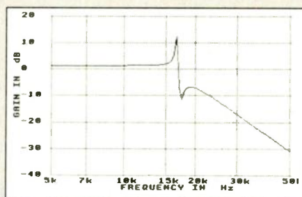
Fig. 1. Original steep-cut low-pass filter with notch at 19kHz.
