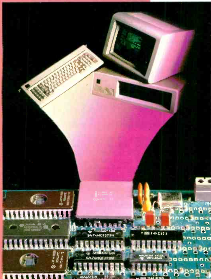
CPU. Reality is that the PC performs the compiling and interpretative functions but that all time and I/O critical actions occur on the target board. (Source: Comsol)
