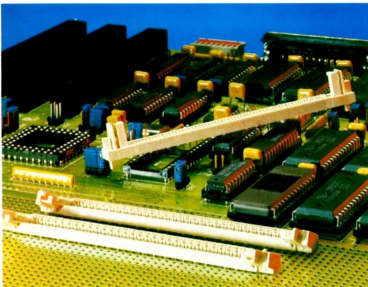
Low profile: AMP SIMM connectors protect your modules while you're changing.
