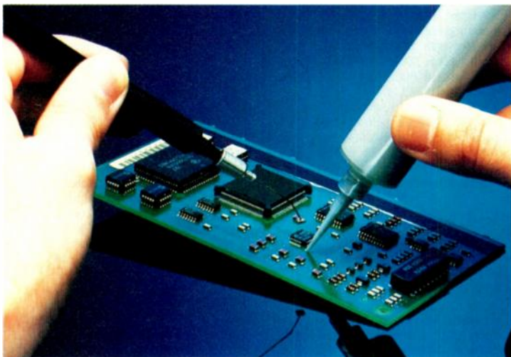
Suck it and flee: the VPP803A vacuum pick up and place tool for small parts.
