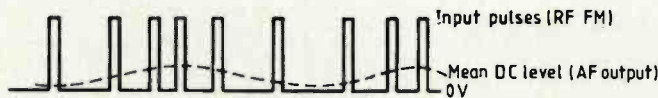
Fig. 5. Pulse-counting FM demodulator. Pulses are derived from FM signal, AF output being proportional to average level and therefore frequency.
