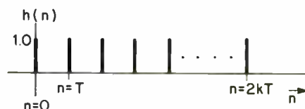
Fig. 5.32. Computational efficiency is achieved by expressing the truncated impulse response (a) as the difference between the IIR (b) and weighted/delayed IIR (c).
