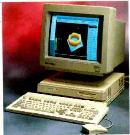
Acorn's R260 - with Arm 3 risc processor, 100Mbyte disc drive and up to 16Mbyte ram.
