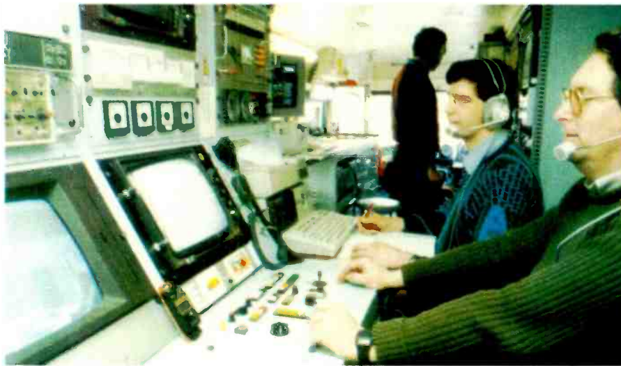
Existing ground control station for unmanned aircraft at the RAE. The new design will include better displays and allow the operator faster and more complete control.
