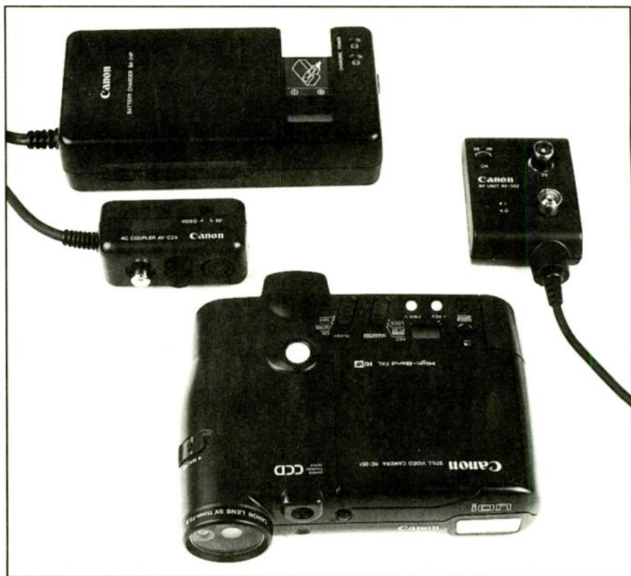
ION, Canon's Hi-band-only SVC with RF unit, AC coupler and battery charger.
