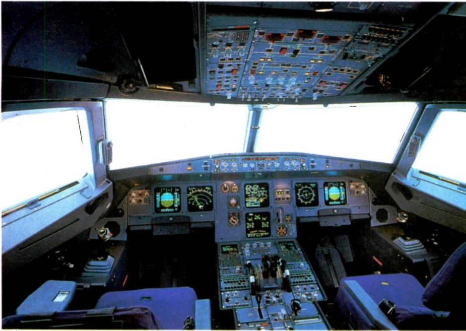
Fig. 1. A320 flight deck, showing the two sidesticks. Cockpit is for two crew, all "lateral" system controls being accessible to pilots
