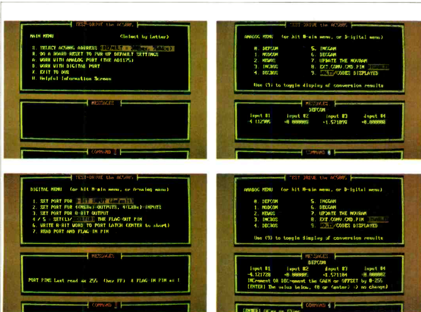
Fig. 1. Main menu and selection of menu screens associated with the evaluation board. The software includes a Basic source code listing for customisation to individual specifications. There is also a help screen file for use with .EXE code, and a conversion program.
