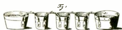
Volta's "crown of cups" - pairs of dissimilar metals with each end dipped into goblets containing brine.
