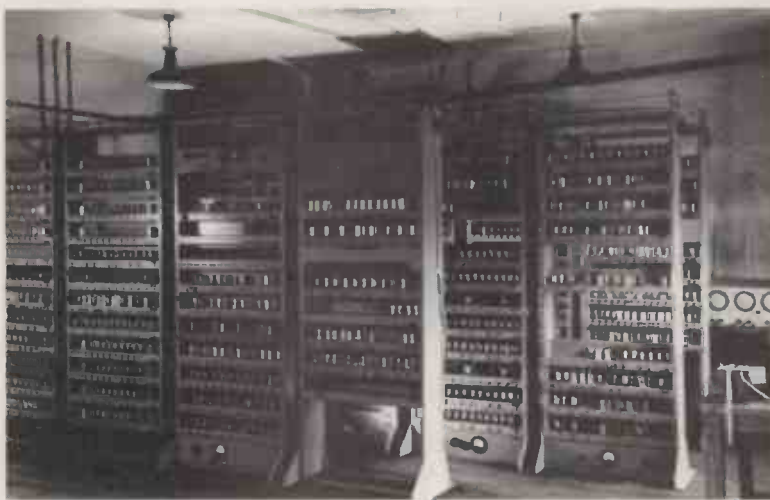
Edsac, circa 1949 – the first computer to run a program read into memory.
