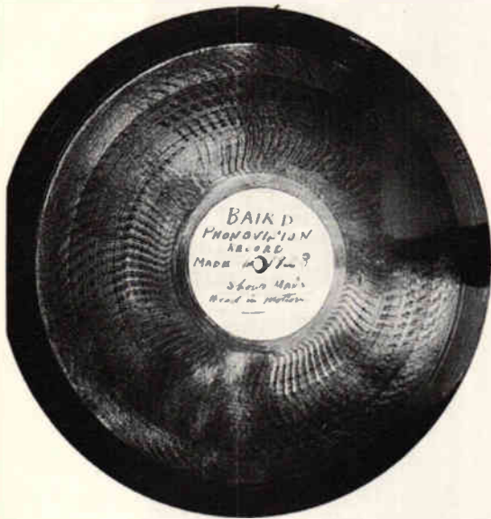
Fig. 1. The Phonovision discs all resemble 25cm (10in) diameter single-sided 78rev/min 'shellac' audio discs. A distinguishing feature is the radial structure caused by Baird's synchronous recording method.
