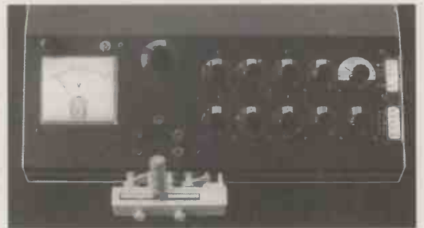
Photo 1. Based on the circuits in Figs 5 and 6, this bridge has independent balancing arms. Its variable capacitance arm measures esr, the variable resistance arm measures capacitance over nine ranges, to a maximum of 1F. Internal switching provides three inductance ranges to 100mH. Two capacitor connection methods, Hewlett Packard test jigs or four terminals with guard lead wires, can be seen.
