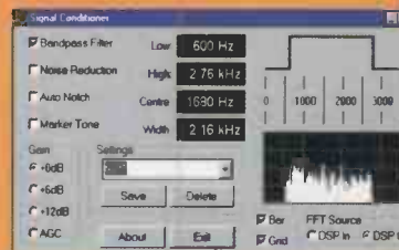
The DSP applet provided with the WR3000 allows continuous control of audio bandwidth and other signal conditioning functions
