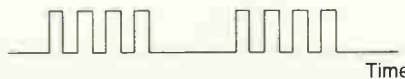
Fig. 6. Output waveform of the Kenwill Smart Charger switches between 4.8V and 1.5V at a 50Hz repetition frequency. Its peak current is about 60mA.
