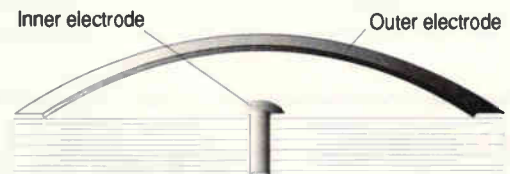
Fig. 3. Developed from the basic multilayer, this discoidal construction provides high capacitance in a small size. The lead-through centre hole and multiple grounded electrodes ensure electrical screening from top to bottom faces.
