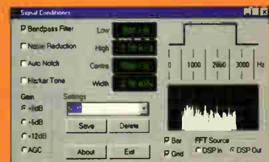
The DSP aspect provided with the WR3000 allows continuous control of audio bandwidth and other signal conditioning functions
