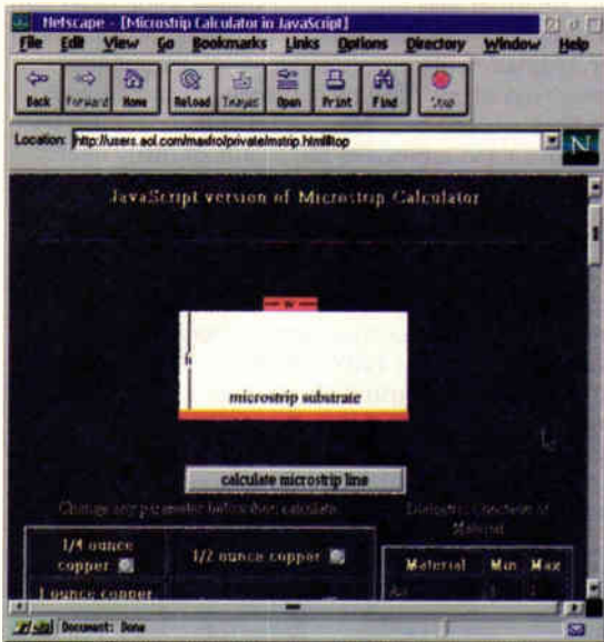
Fig. 7. Design microstripline widths/impedances on-the-page. Another unique Max Froding rf utility.
