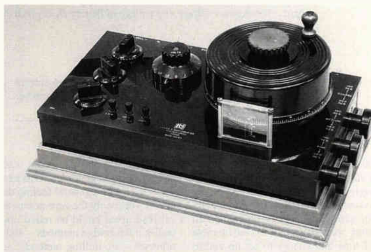
This Leeds and Northrup version of the potentiometer is an adaptation of the Crompton arrangement, one of a series (K1 through K5) sold as recently as the 1980s. This one is a K2, dating about from the 1940s. It has three ranges, with full-scale readings of 1.6V, 0.16V and, believe it or not, 0.016V.
