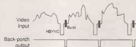
Fig. 6. For horizontal sync, the 4881's back-porch signal is used. At 2.5 \mu s, this pulse is just wide enough for the 6145 display chip.
