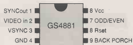
Fig. 5. Pin compatible with the industry-standard LM1881, the GS4881 extracts horizontal and vertical sync signals from composite video.
