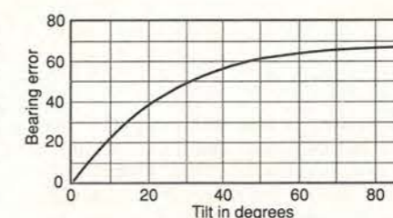
Fig. 2. Bearing error versus tilt angle shows how error rate increase with tilt gets smaller as the tilt increases.
