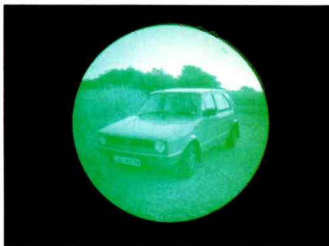
Moonless night, but under open sky. The naked eye could resolve the outline of a vehicle but no details. The light in the sky is reflected from a town some ten miles distant.
