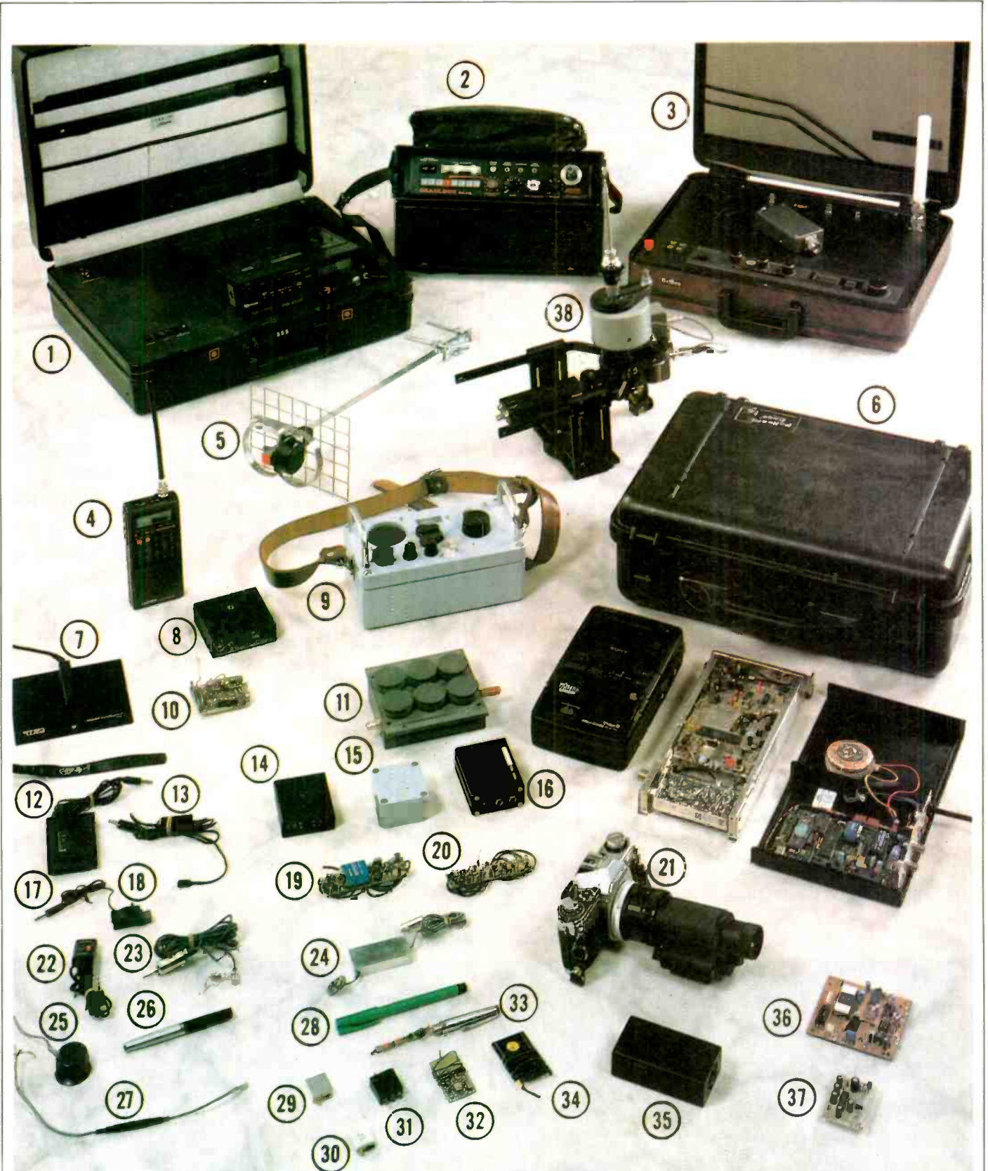
A selection of devices available to the well equipped spy. (1) old-style video recorder and camera in a briefcase; (2) Scanlock bug detector; (3) video and sound microwave receiver in briefcase with 1.4GHz masthead preamp, radio control built-in; (4) scanner receiver; (5) 1.3GHz "how-tie" antenna; (6) new video and sound receiver using Sony Watchman and a variable-bandwidth 950-1750MHz PLL tuner; (7) Pressure Zone microphone; (8) and (10) single-channel VHF receiver; (9) simple SSB tracking receiver; (11) heavy-duty pulse target tracker; (12) PZ microphone; (13) body-worn microphone; (14) FM radio microphone; (15) personnel target tracker; (16) low-cost microwave TV transmitter; (17), (18), (22), (23) commercial lapel microphones; (19) parallel telephone transmitter; (20) series telephone transmitter without battery; (21) Canon camera with M911A night-vision lens; (24) Mullen 100mW body-worn VHF transmitter; (25) sucker microphone; (26) phantom-powered line pre-amp; (27) line amplifier; (28) target tracker transmitter in a pen; (29), (30) Gem VHF and 1.1GHz 100mW and 20mW body, room and telephone transmitters; (31) infrared target tracker; (32) "visiting card" audio VHF transmitter; (33) Wild (1970) VHF pen transmitter; (34) "visiting card" tracker transmitter which responds to light; (35) TV camera with motorized auto iris; (36) scrambler module; (37) video AGC unit for long cable runs; (38) Antenna Eye main unit.
