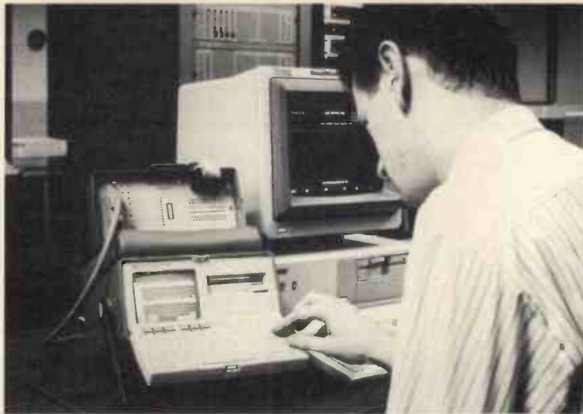
Hewlett-Packard 4951 protocol analyser for 19.2 kb/s data communications.
