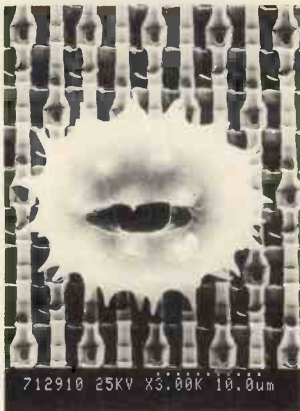
The picture shows the 1µm structures on Siemens' latest 1MB DRAM chip compared to a pollen grain.
