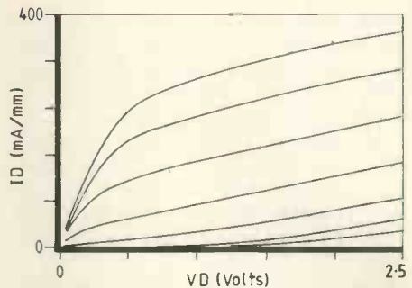
Typical current/voltage characteristics with d.c. drain for a 100 nm by 150 \mu m T-gate Modfet.
