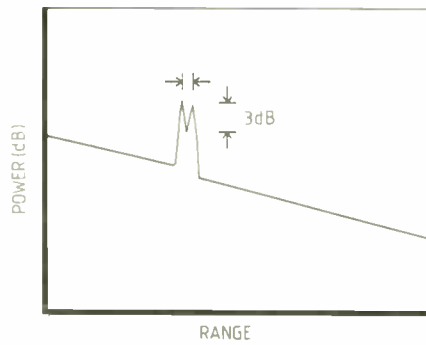
Fig.5. Response resolution is the minimum separation at which two faults can be distinguished from each other.
