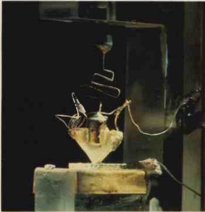
Fig.2. The first point-contact transistor, 16 December, 1947 (photograph by courtesy of Bell Laboratories).
