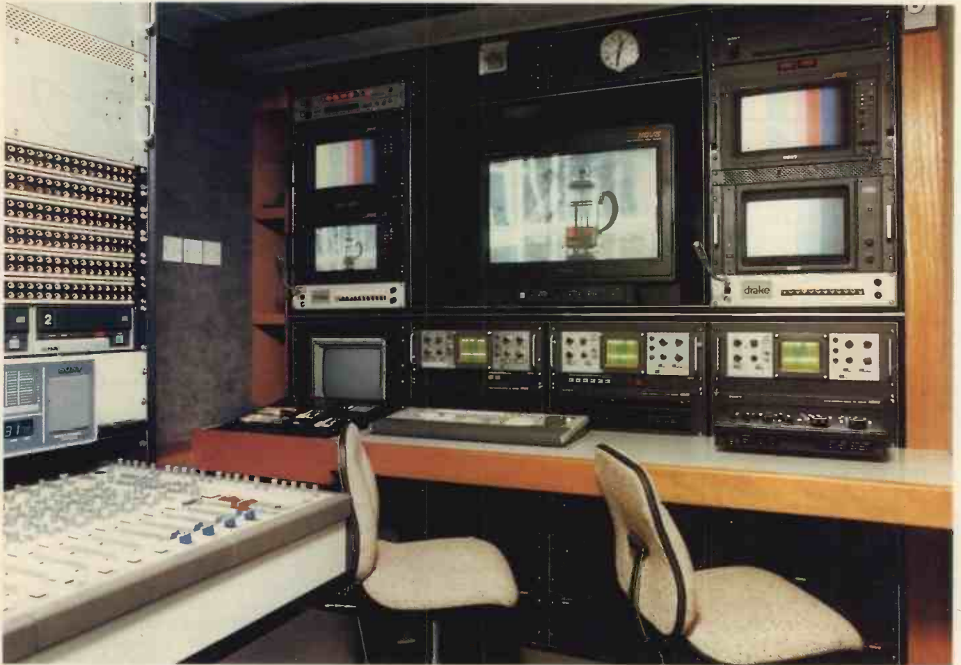
This suite of high-definition production equipment by Sony is based on the Japanese 1125/60 format adopted by NHK.
