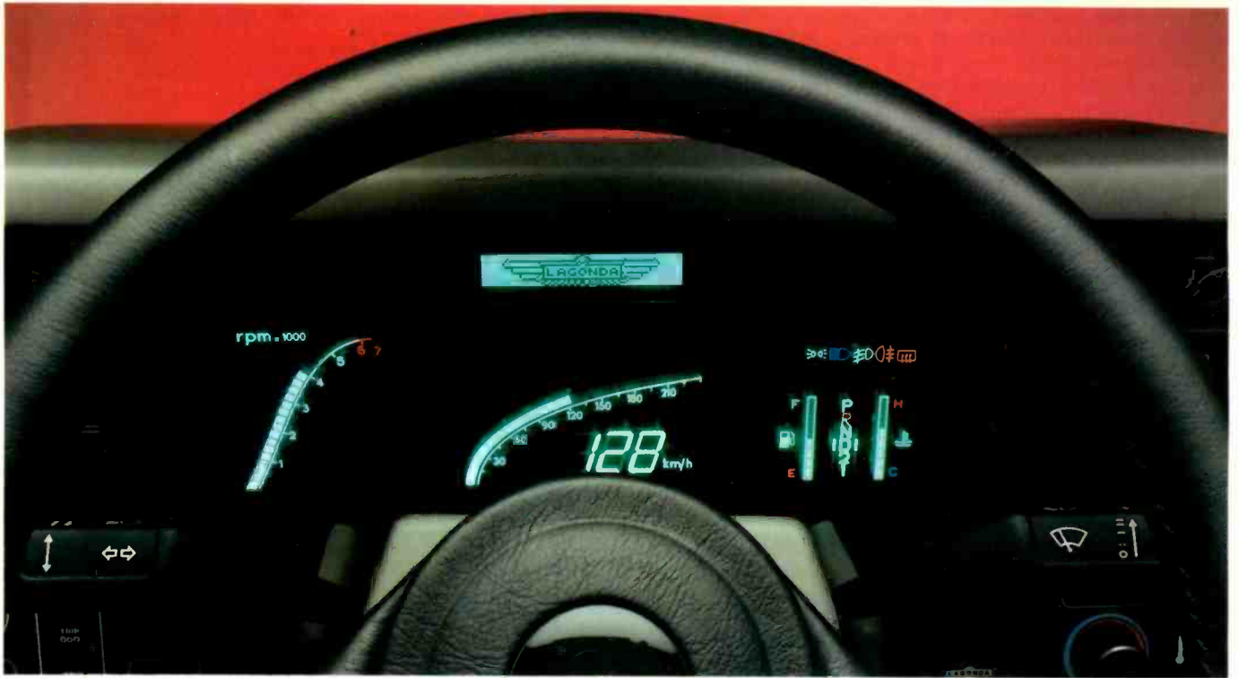
This vacuum fluorescent display dashboard was designed for the Aston Martin Lagonda, by Kemitron. Road and engine speed r.p.m. are shown on bar-graph gauges, all the usual standard warning symbols are incorporated, and a separate dot-matrix display is linked to a speech synthesizer to give system messages.
