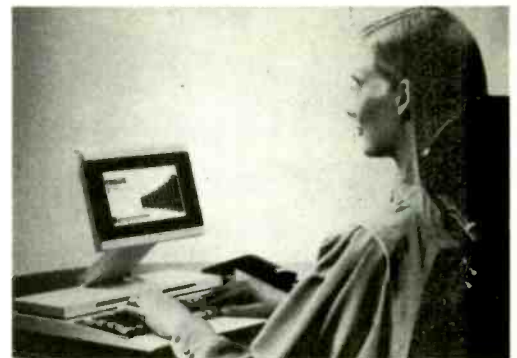
Intended for use in portable computers but also suitable for laboratory instrument applications, this electroluminescent display comes from Finland (Lohja corporation). It has all the electronics necessary to be compatible with the output of an MS-DOS computer.
