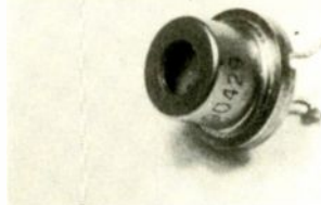
Fig.2. A Sharp LT022MC GaAlAs laser diode package. This relatively low-cost device is found in many compact disc players.
