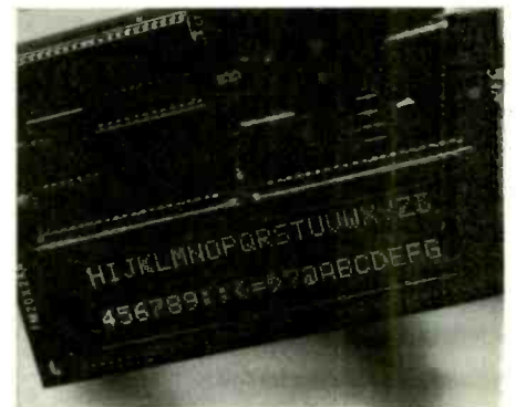
This fluorescent indicator from NEC includes all the support and control electronics to allow the unit to be connected directly to the data and control signals.
