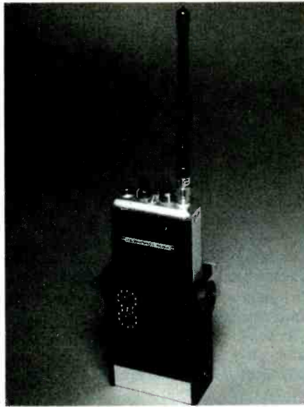
The Tele-Niros v.h.f. hand-portable is supplied with up to four channels and with open or selective calling (Tele-Nova Ltd).
