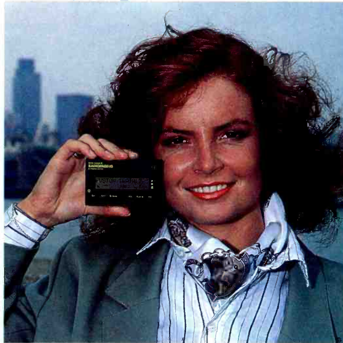
Messages up to 90 characters long can be received on this display pager, which has a memory capacity of 512 characters. A built-in clock time-stamps each item.
