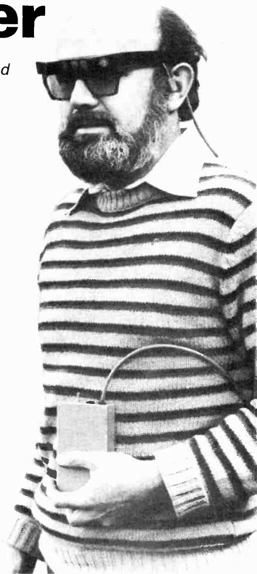
Fig. 1. Dr Heyes wearing a prototype of the Sonic Pathfinder.
