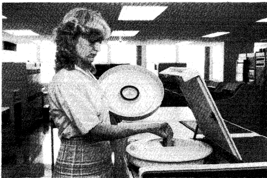
A cartridge being loaded into a drive. The cartridge base cover is stored on top of the cartridge to keep it clean.
