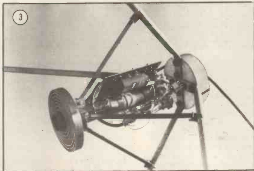
Fig. 1. Sheffield terminal's 8ft dish antenna with 4GHz feed in position. Fig. 2. 4GHz head unit. The GaAs f.e.t. stage is mounted near the top. Fig. 3. 11-12GHz feed system mounted at the prime focus point.
