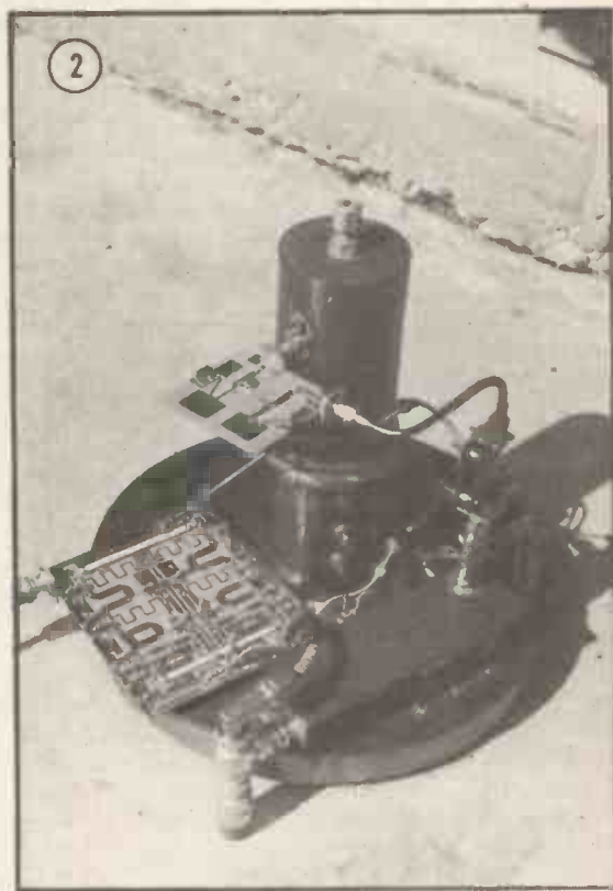
Fig. 1. Sheffield terminal's 8ft dish antenna with 4GHz feed in position. Fig. 2. 4GHz head unit. The GaAs f.e.t. stage is mounted near the top. Fig. 3. 11-12GHz feed system mounted at the prime focus point.
