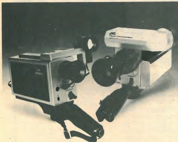
A low-cost colour camera to match growing needs: the basic JVC G31P accepts options like a more versatile lens and electronic viewfinder.
