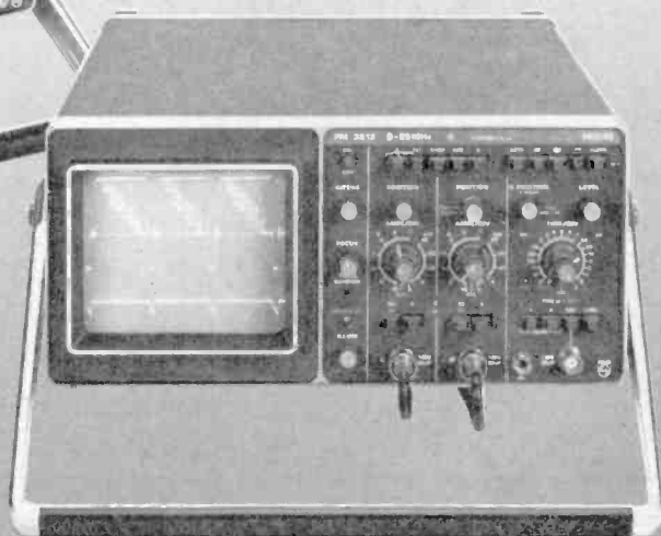
PM 3212: 25 MHz/2mV. Dual-trace. Comprehensive triggering facilities including peak detected auto mode, d.c. coupling, t.v. sync and composite.
