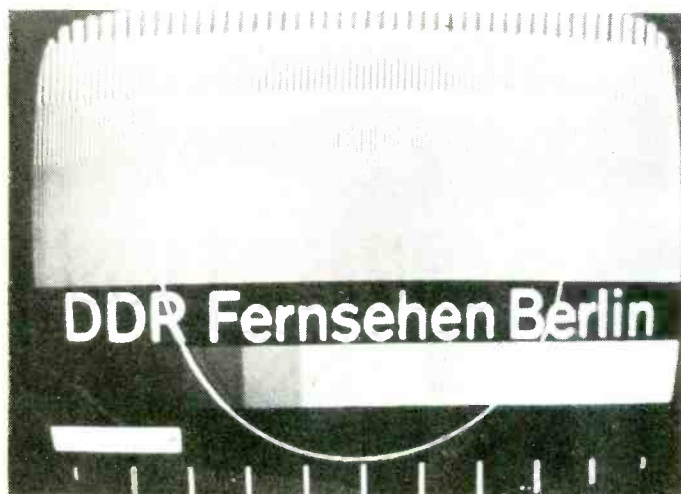
East Germany DDR-F (B, G) SECAM colour — There are several different identifications used with this electronic test card.
