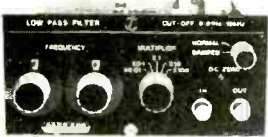
EF3-02 Low Pass Cut-off frequency variable from 0.01Hz to 10kHz
