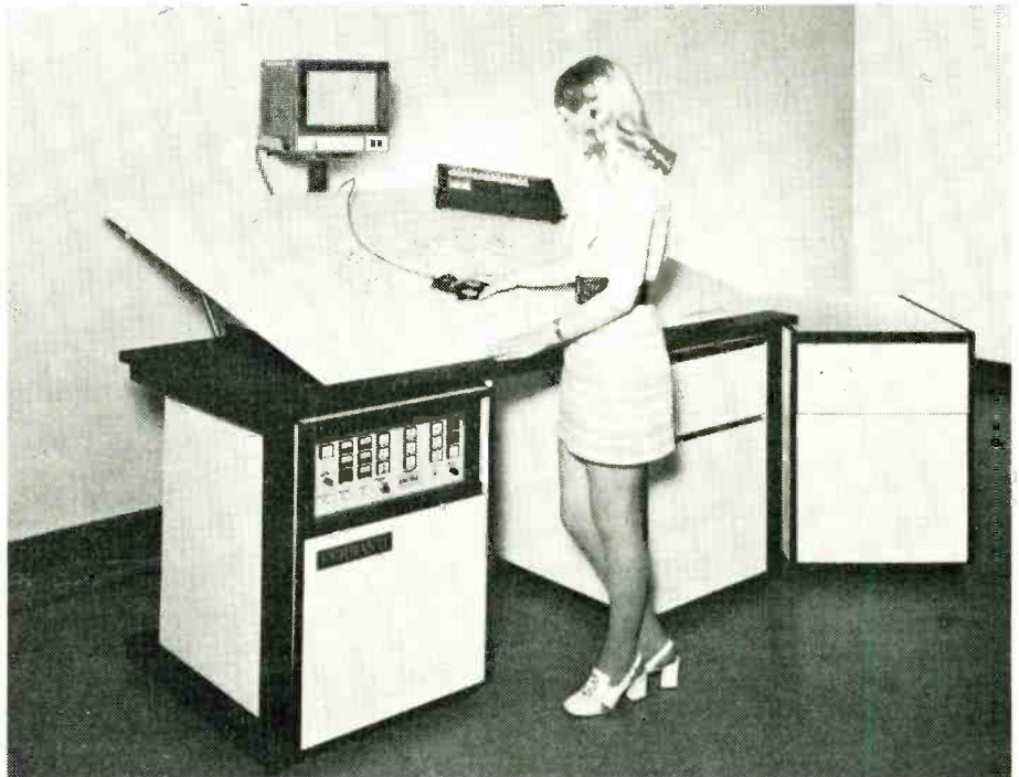
The Ferranti Feedraft used to automatically generate p.c. masters, i.c. masks and other drawings.
