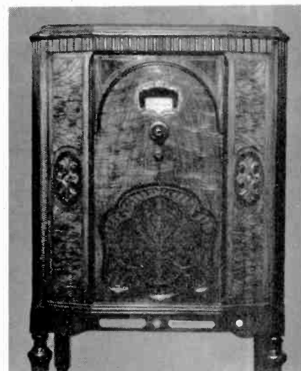
1930: Brunswick (U.S.A.) model 15, illustrating "furniture" approach in console cabinet design; t.r.f. circuit; four screen grid valves in r.f. and detector stages, with 4-gang capacitor; two triodes in parallel for a.f. Loudspeaker energizing coil acts as a.f. choke in anode circuit; audio signal via capacitor to output transformer. Good sound quality with pronounced bass response.
