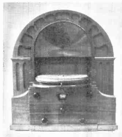
c.1933: Micro-Perophone table radiogram (minus pickup). Regentone superhet chassis. Compact synchronous motor (not self-starting), windings mounted on underside of motor board, which is hinged and folds downwards. Speaker behind metal casing enclosing turntable, sound being reflected through front ports around periphery of cabinet.
