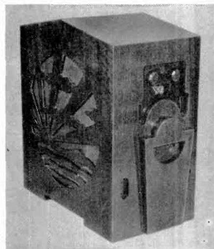
1931: Pye "transportable" MM, weighs nearly 40lb. Three-valve plus rectifier t.r.f. mains set. Built-in frame aerial (set tuned for maximum signal pick-up and selectivity). Two-gang tuning covers m.w. and l.w. Fine tuning trimmer capacitors across aerial section of ganged capacitor. Moving-coil loudspeaker.
