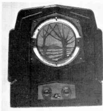
1932: Ekco SH25 superhet. Selectivity allows station names on dial surrounding speaker. 110kHz i.f. and 110kHz aerial filter; bandpass aerial tuning; pentode frequency change/biased as anode bend detector, oscillator voltage to cathode; "local/distant" switch introduces damping in i.f. (no a.g.c.); volume control adjusts i.f. valve bias and aerial circuit damping; control for cancelling second channel; pickup sockets.
