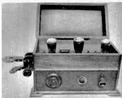
Mid-1920s: 3-valve receiver, probably made from a kit. Note the swinging reaction coils on outside of mahogany case.
