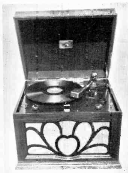
1931: H.M.V. 501. 3-valve plus rectifier t.r.f. table radiogram. Three-gang tuning, bandpass aerial circuit, series aerial trimmer (control on side) and reaction (control on other side). Illuminated dial on motor board. Pickup tracking weight 200 grams. Lid has felt lining to reduce mechanical noise. Power unit has resistive smoothing – probably reason for some mains hum.
